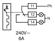
. (terminals marking on the  $2^{nd}$  CA are 21 / 22 / 24 when the selector of the reference 4 062 64 is in the "CA" position).
